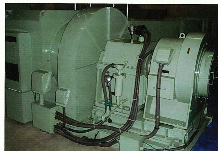
Horizontal assembly bearing for Water turbine
